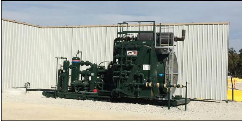
**FIGURE 15.2** Gas compressor. (Source: © energy.fanchi.com (2015).)
