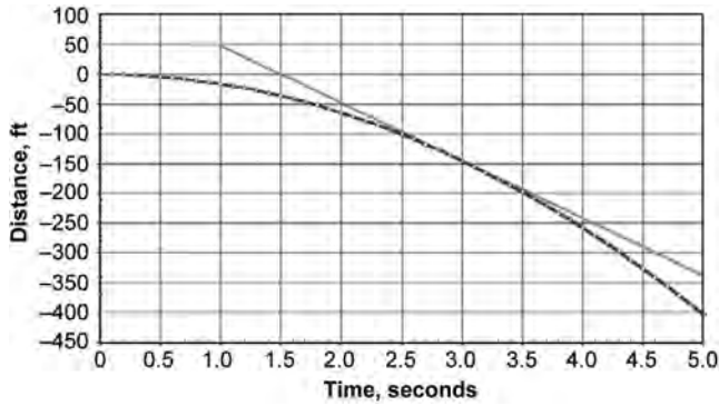
Fig. 1.1—Graph of Eq. 1.1, the equation of free fall on earth.
